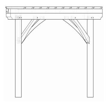
The Little Gull is a triangular pergola designed for tighter spaces or corners. It is precision fabricated on advanced CNC machinery using the highest quality Douglas fir timbers. Wood-on-wood joinery provides a timeless aesthetic and allows for easy installation. This product is delivered in kit form with numbered parts, drawings, wood pegs and fasteners. This product requires assembly by an experienced carpenter with timber frame knowledge.
